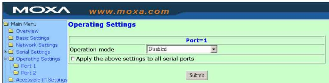
When Operation mode is set to Disabled, that particular port will be disabled. Check the "Apply the above settings to all serial ports" to apply this setting to the other port.
