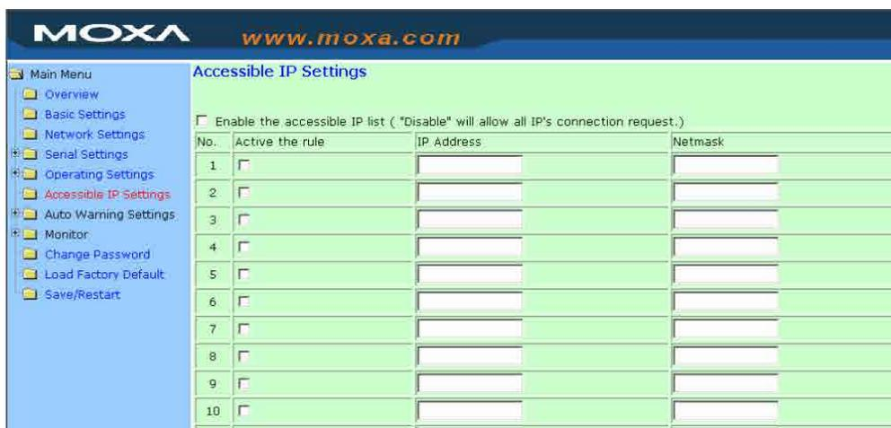
The NPort 5100 uses an IP address based filtering method to control access to itself.
