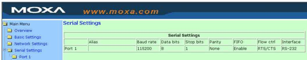
To modify serial settings for a particular port, click either **Port 1** under **Serial Settings**, located under **Main Menu** on the left side of the browser window.
