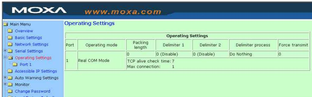
Click **Operating Settings**, located under **Main Menu**, to display the operating settings for both of NPort 5100's serial ports.
