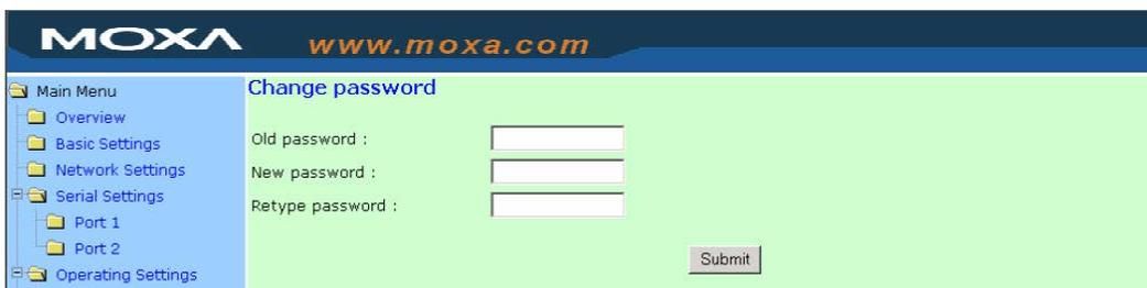
Input the "Old password" and "New password" to change the password. Leave the password boxes blank to erase the password. If the password is erased, then NPort 5100 will not have password protection.
