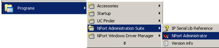
2. Unlock the NPort 5100 you wish to configure if it is password protected. Right click the NPort 5100 and select **Configure** to start the configuration.
