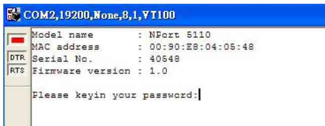
9. Start configuring the IP address under **Network Settings**. Refer to step 4 in the **Telnet Console** section for the rest of the IP settings.
